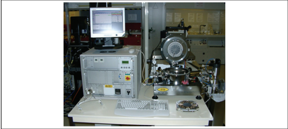
Fig. 6. Wafer bonding: EVG bonding machine used for wafer pre-bonding (the bonding is finished using a classical press)
